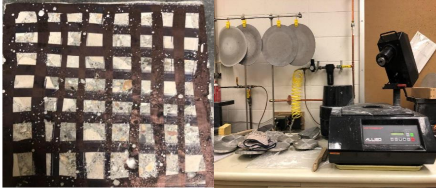
(a) Sample drawn with orthogonal grid (b) Polishing disk and machine
